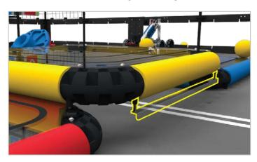
Figure 11: A close-up view of the Center Platform, with the polycarbonate structure underneath highlighted. This structure's intent is to keep Balls out from underneath the Center Platform per <SG9>; it cannot be used for Parking.
