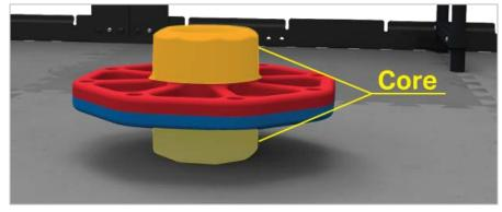
Figure 7: Close-up of Cap, with the Core highlighted.
