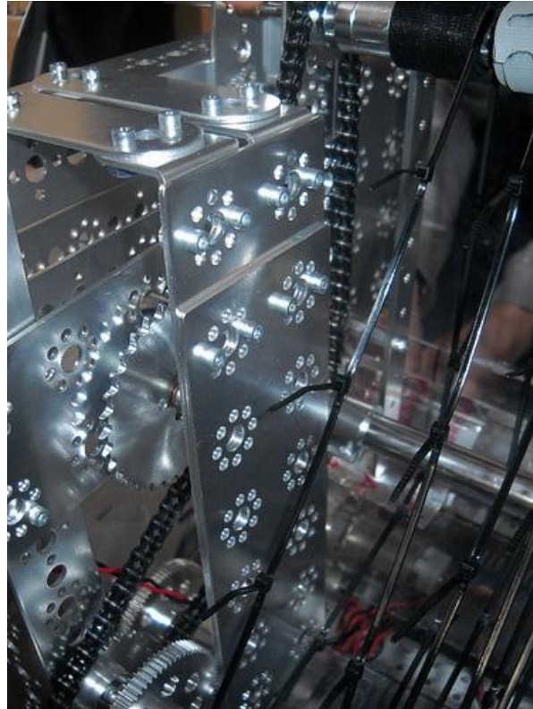
Figure 100: Tension Sprocket Addition
