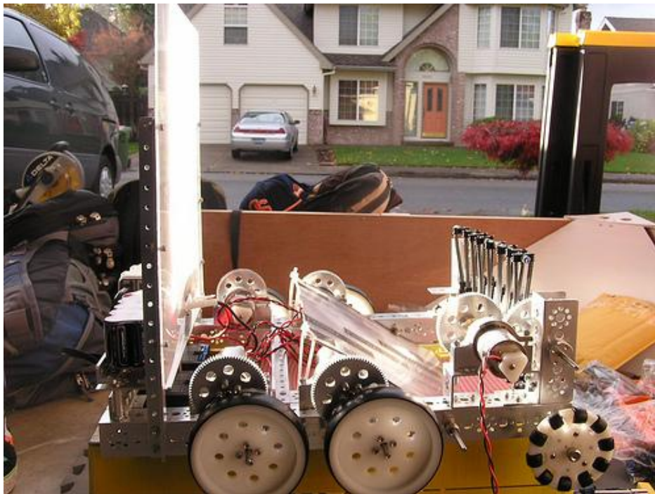
Figure 31: Ball Transport and Storage Concept (Side View)
