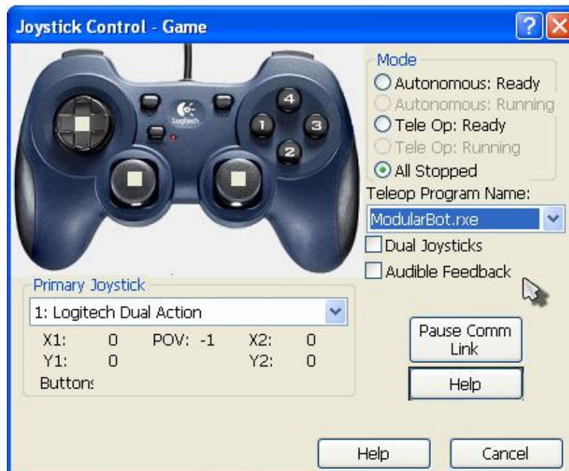
Figure 36: Correct Teleop Setup
