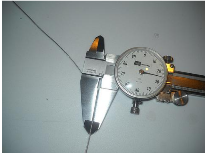
Figure 89: Micrometer Measurement of Plastic Coated Rope
