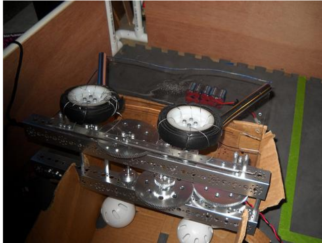
Figure 96: Ball Shooter Guiderails under Test
