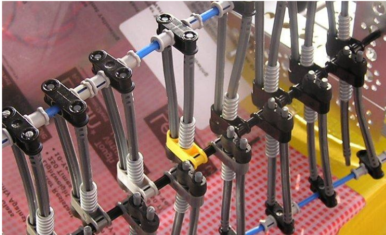
Figure 41: New Ball Collector with Flexible Rods (Close-up)
