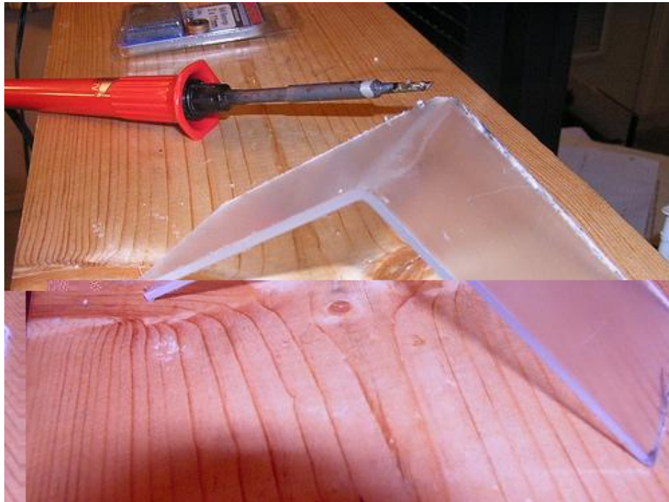
Figure 33: Solder Iron Plexiglas Bend Method
