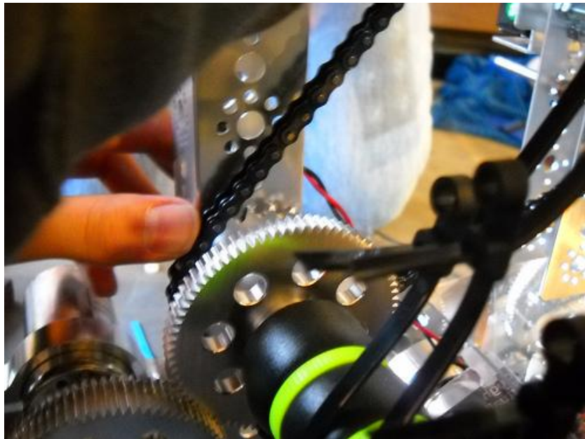
Figure 93: Chain being mounted on sprocket
