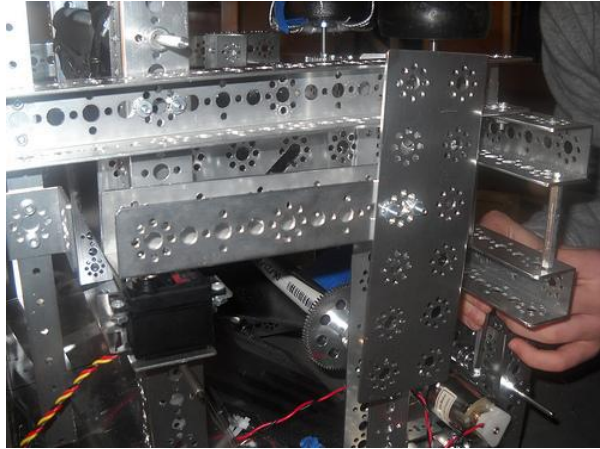
Figure 74: Right Side Servo Mounting
