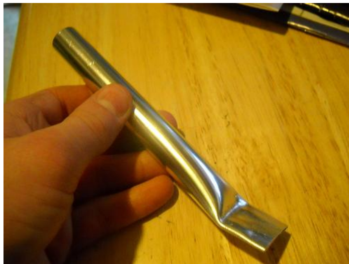
Figure 95: Completed pressed tube end to fit under ball shooter tires
