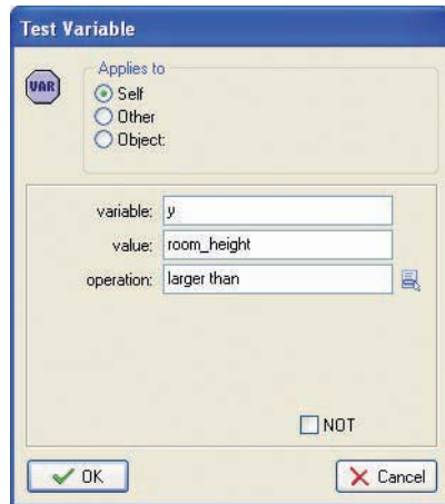
Figure 9-2. This action tests whether the island is below the visible edge of the room.
