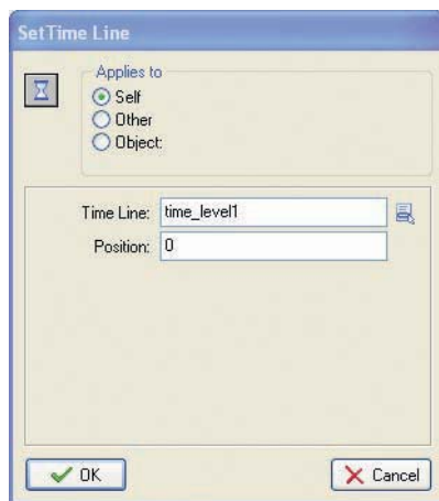
Figure 9-6. The Set Time Line action is used to start a time line.
